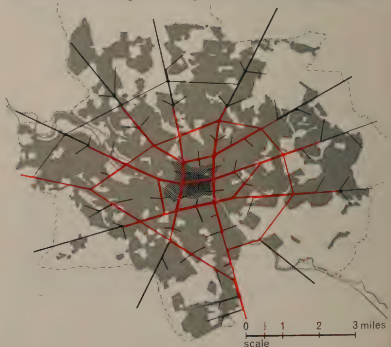
121 The theoretical intermediate network which would meet about 40% of the potential demand for travelling to work by car in the central zone. The distributors shown in red would need to be built to motorway standards.
